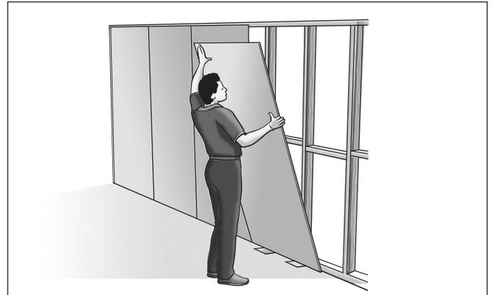
FIGURE 4 SHEET INSTALLATION
