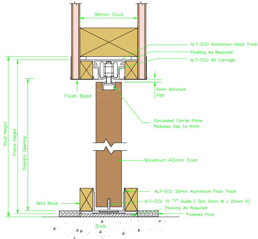
Detail 6 | Metinno Flushline Full Height Detail
