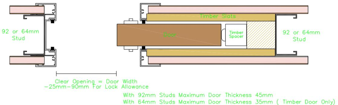
Plan View with Aluminium opening frame. Available for 64mm and 92mm steel studs.
