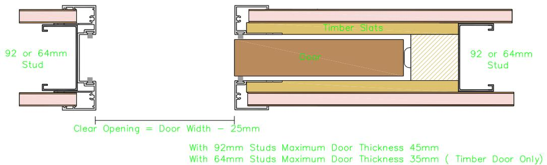
Detail 18 | Metinno Aluminium Clear Opening with Lock Allowance
