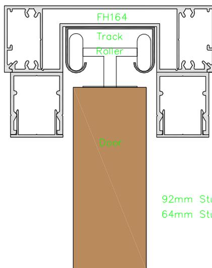
92mm Studs Maximum Door Thickness 45mm
