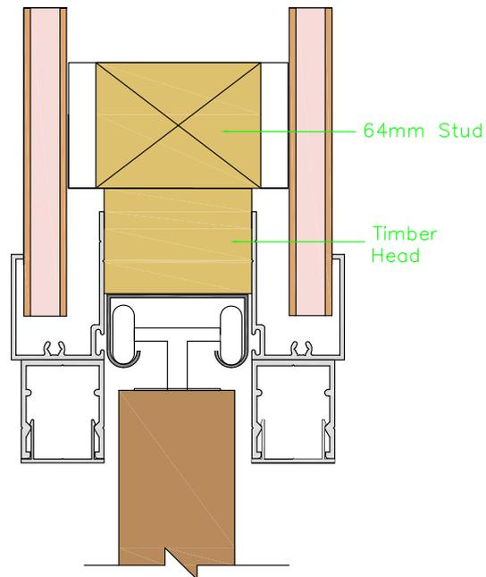
Detail 19C | Metinno Aluminium Receiver to Partition
